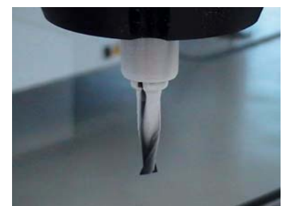
Tool, cooled by CoolMin internal
