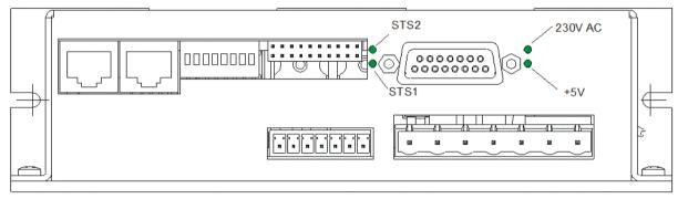
Via the LEDs on the front, it is possible to indicate the existence of the two main supply voltages. Furthermore, the current state of the module can be viewed here (STS1 and STS2)
