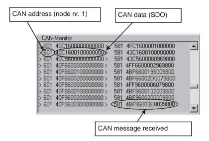
In this window, CAN data are shown which are exchanged between the ACSetup programme and the selected drive module.
