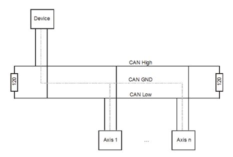
For the CAN wiring, it is recommended to use twisted shielded cables with a characteristic impedance of 108 to 132 ohms. In case of very small network extensions, it may be possible to dispense with the connection of the reference potential (CAN ground) (not recommended).
