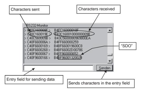
Here, all data are shown that are transferred via the serial interface (RS232). The characters sent are marked with two arrows by the ACSetup programme. Characters received are written behind this.
