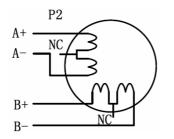
6-lead motor half coil (higher speed) connections
