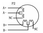
6-lead motor half coil (higher speed) connections
