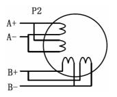
8-lead motor parallel connections
