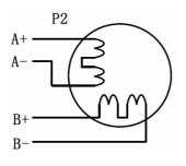
4-lead Motor Connections
