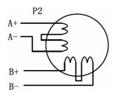
8-lead motor series connections
