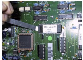
Take the first memory module, labelled "IMC4 V2.4.00 high", out of the protection box and insert it into the horizontal socket () on the right side of the processor (square socket) in such a way that you can read the writing on the label. In this case, a groove in the case of the memory module is visible on the left side of the socket (PIN 1, horizontal lower left side). While performing the described process, make sure you don't bent a PIN of the memory module.
