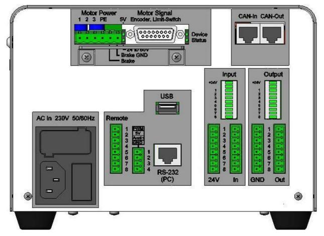
Image 5: Back side view controller MC1-30
