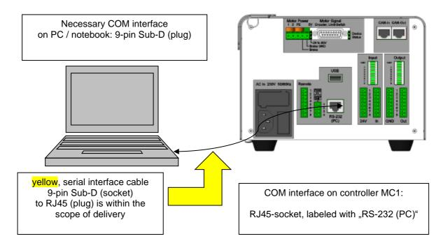
Image 7: Serial connection (RS232) via interface cable of PC / Notebook to MC1
