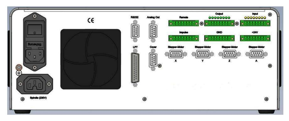
**Stepper-Motor connector** – motor axis X-, Y-, Z-, A, Sub-D9-pin socket SubD-9-pin connector for motor modules (CNC axis)
