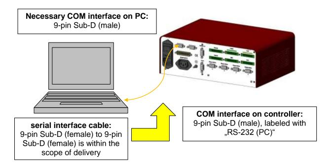
Image: serial connection (RS-232) between PC / Notebook and iMC-P via interface cable
