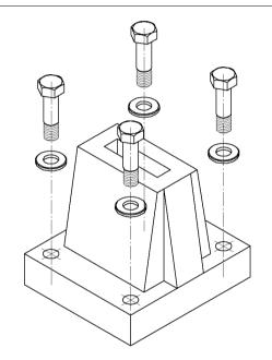
When designing in the exploded view the explsion axes can be inserted as 3D lines to improve the claroty of the 3D views, in particular the parallel perspectives.
