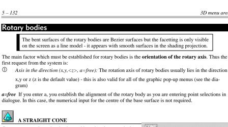
Generate a cone through selection and by using the numerical pop-The tip of the cone lies vertically above the centre point.
