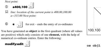
You will now find yourself in the Editor which shows the geometrical data for the stored lines. isy needs six internal commands in order to generate the object, which you will only seldom be confronted with when you are entering co-ordinates using the mouse. isy stores all drawings in the vector directory using this alphanumeric form. The short commands which are used here have the following meanings
