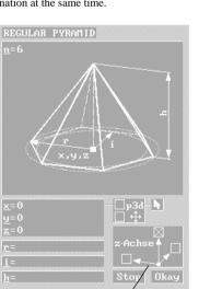
Orientation of the central axis Alignment of the object in the x,y,z directions (z is pre-set)
