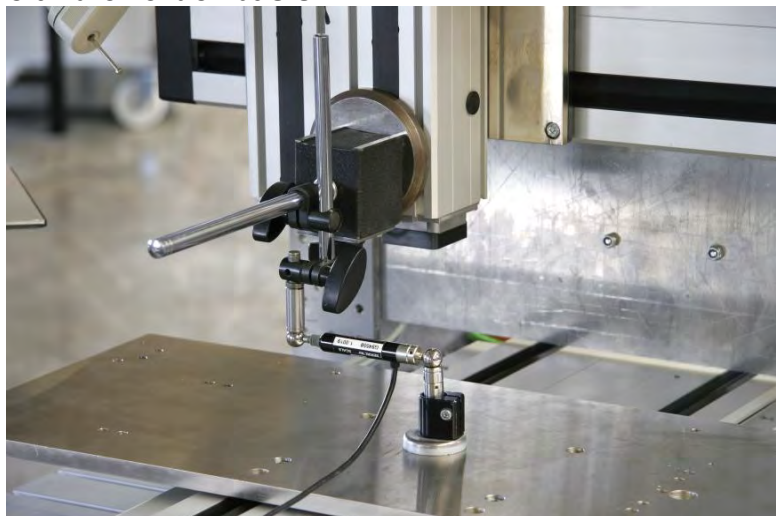
Figure 4: Circularity measurement with the Renishaw QC10 circularity measuring system
