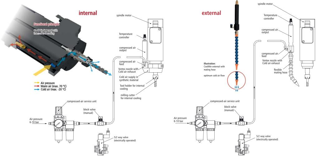
The isel tool cooling system is operated with cold air (up to max. -20°C). In this system, normal operating air (6 up to 10 bar) is used and is freed of dirt particles with a compressedair service unit to prevent icing.
