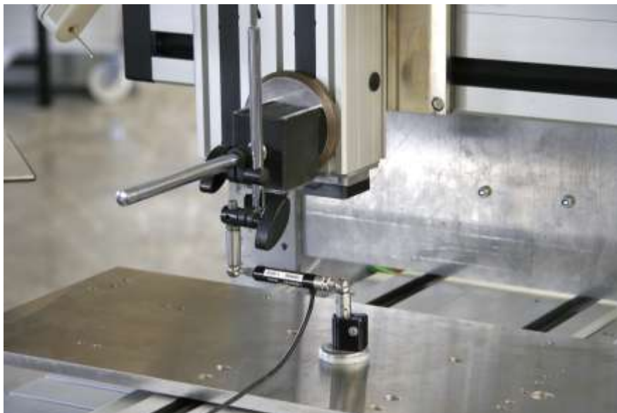
Picture: circular form measure with Renishaw QC10
