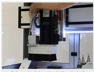
Option: suction device equipped with suction head
