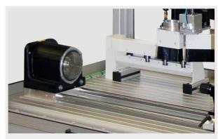
Option: rotation unit, RDH series, can be integrated as a 4th axis
