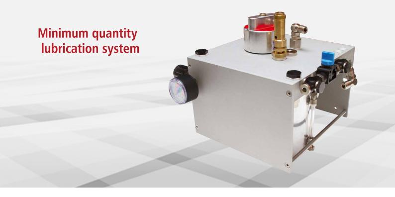
The minimum quantity lubrication (MQL), also called minimal quantity cooling lubrication (MQL) works according to the principle "less is more". A cooling lubricant-air mixture is used to prevent the generation of frictional heat through optimal lubrication. The remaining heat is dissipated through the tool and the chip.
