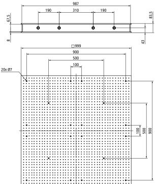
The workpiece can be clamped very rapidly by switching the chambers and covering the remaining bores around the workpiece through the vacuum distributor (4-fold or 8-fold) with pressure monitors. The open bores of the switched clamping chambers are closed with an adapter mat. Our rotary vane vacuum pumps are suitable for the generation of the vacuum.
