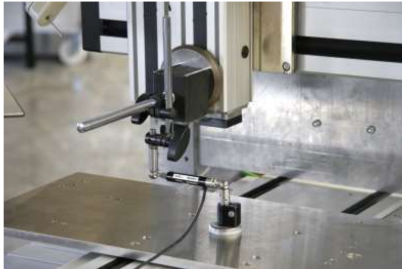
Figure: Circularity measurement with Renishaw's QC10 circular form measuring system
