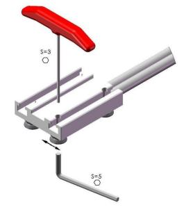
Repeat this process until the slide runs backlash-free and smooth-running. After a run-in phase of the slides, the bias may be decreased as a result of normal deterioration depending on the load profile and the environmental conditions
