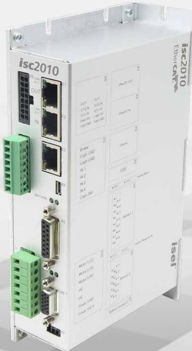
The new universal servo controller **isc2010** with dual multi-encoder interface for permanent magnet synchronous motors, torque motors and linear motors. Power range of 1.2 kW with a rated voltage of up to 100 V. Very short controller cycle times with the EtherCAT real-time bus system for highly dynamic position applications.
