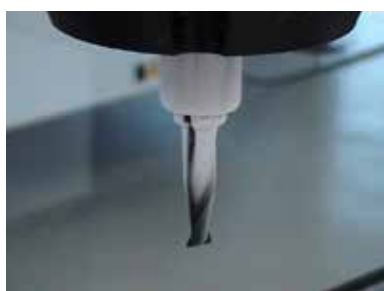
Tool, cooled by CoolMin® internal
