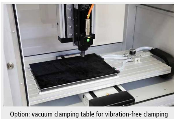
Option: vacuum clamping table for vibration-free clamping
