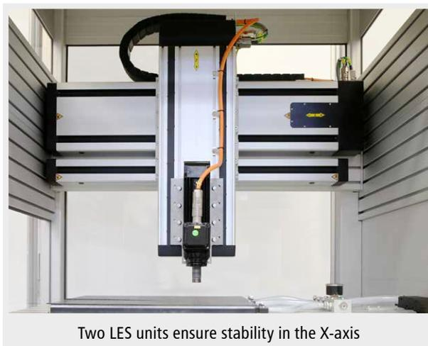
Two LES units ensure stability in the X-axis
