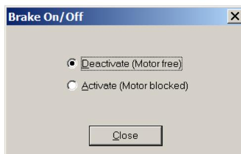
After deactivating the brake, the motors are freely movable. Please do not forget to deactivate both the brake of the master and the brake of the slave. And if you have another vertical gantry axis, you should repeat the same procedure for the other gantry axis.
