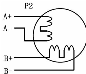
4-lead Motor Connections
