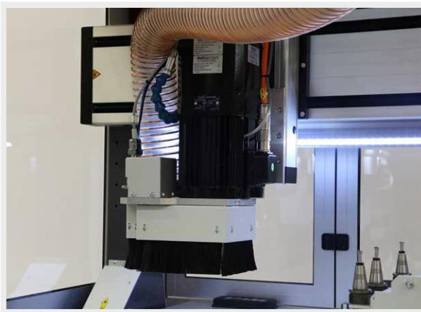
Option: suction device equipped with suction head
