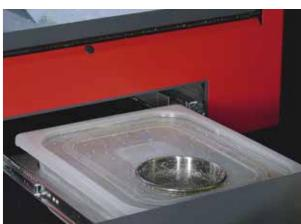
The practical coolant container has a capacity of five liters. For cleaning and filling, it can simply be pulled out and removed through a drawer positioned under the machine. The multi-stage filter system prepares the cooling lubricant for the system cycle by
